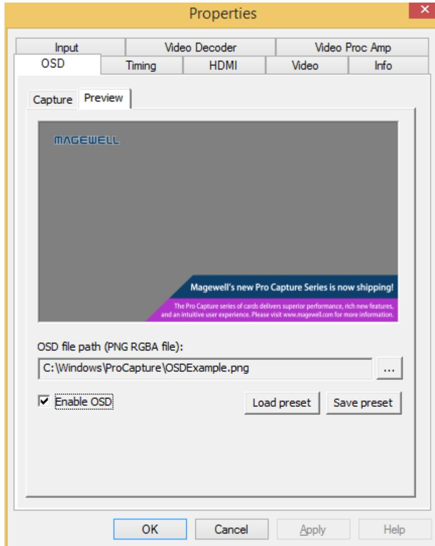
An image with transparency (ie. alpha channel) can be overlaid on the incoming video by using the OnScreenDisplay (OSD) function. Browse to select a suitable 32bit PNG image to use for the OSD. Click “Enable OSD” to activate the overlay. Click “Save preset” to save the current image/path as a template. Users can click “Load preset” to load a previously saved image.
