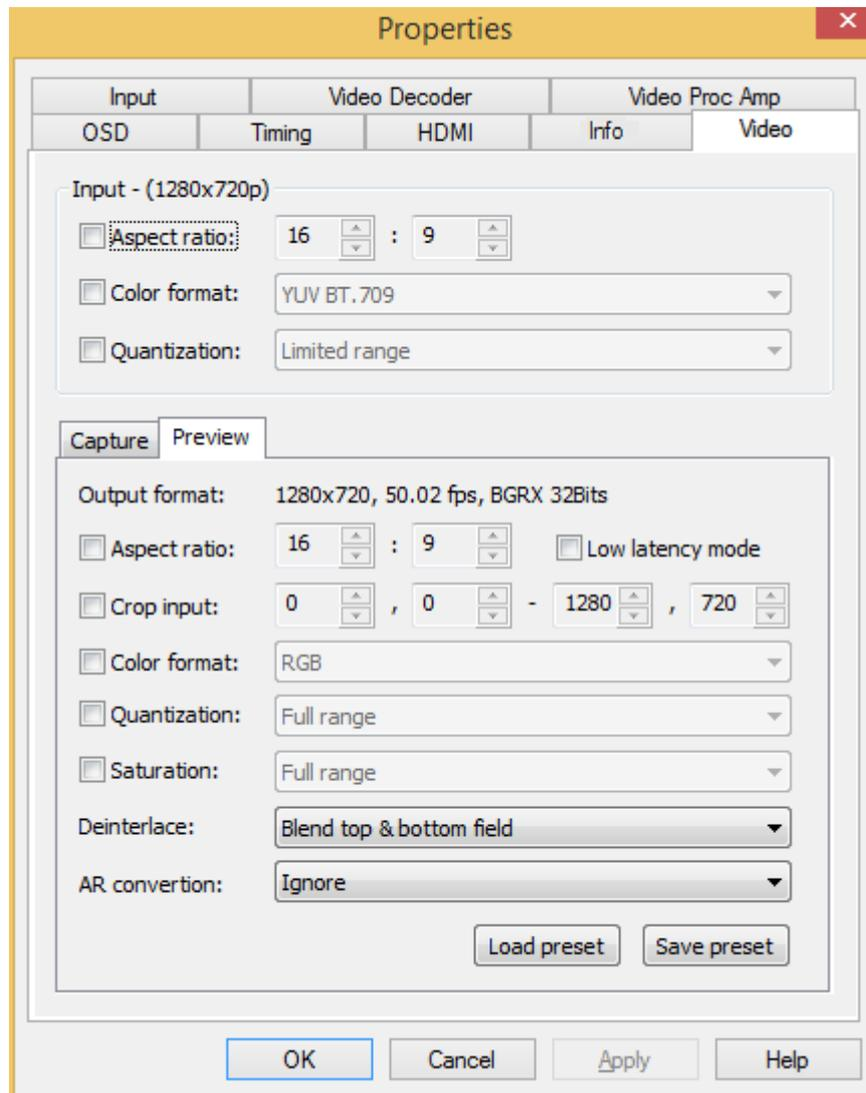
Note : If a box is not ticked, the current related value is shown. If a different value is required, users need to tick the box first and then set the new value.
