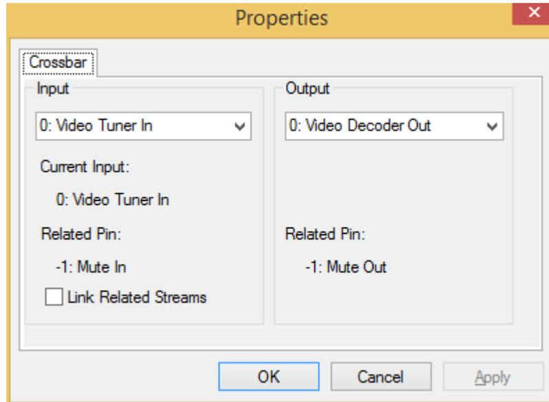
Select a signal type for the “Input” from the drop-down list of options. The number 6 means the current signal, which is auto-detected by the system. When the selected signal is different from the actual input signal, video will not be displayed correctly.
