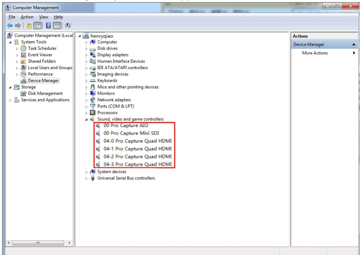
In the device list above, you can see all the capture cards that are installed in this computer. The number before the Pro Capture card name is the ID number of the card. (Eg. 00 or 04 in the example above.) This is the number set via the rotary switch on the card. For multi-channel cards, the channel number will be added after the ID number of the card. (Eg. 04-0 , 04-1 , 04-2 , 04-3 for a Quad card)
